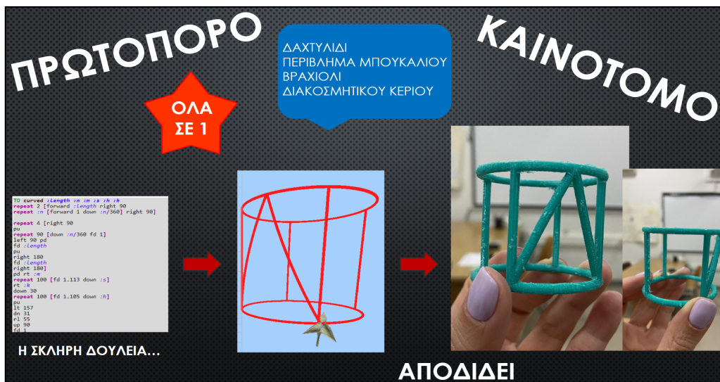
Figure 72: Slide presentation created by students in the DT project “Personalised Items” to promote their product by also presenting the process of its construction (code-digital model-3D printed object) - NKUA0207
